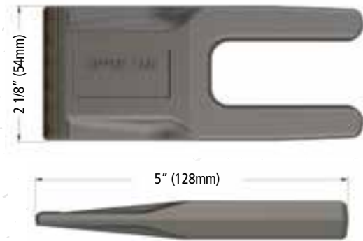
1650 HFFTC Tooth • Abrasive soil • Impact, hard faced with carbide chips on two sides
